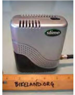
The pump connects directly to your bike's battery with alligator clips, or can plug into a standard electric vest type socket. It had no problem inflating the 190 tire in a reasonable amount of time, although it was a little loud.
