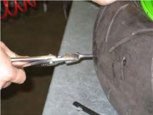
Cut off the excess and you're left with a plugged tire.
