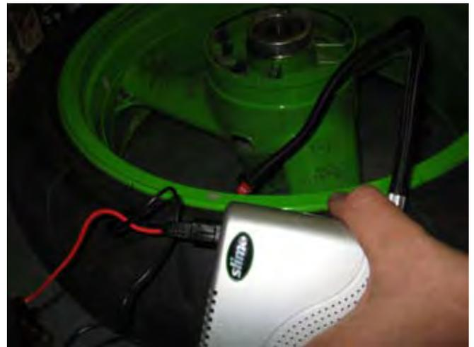
Slime around the inside of the carcass, and to force the Slime into any punctures. We bounced the tire up and down and sloshed the Slime around. Very quickly the leak stopped.
