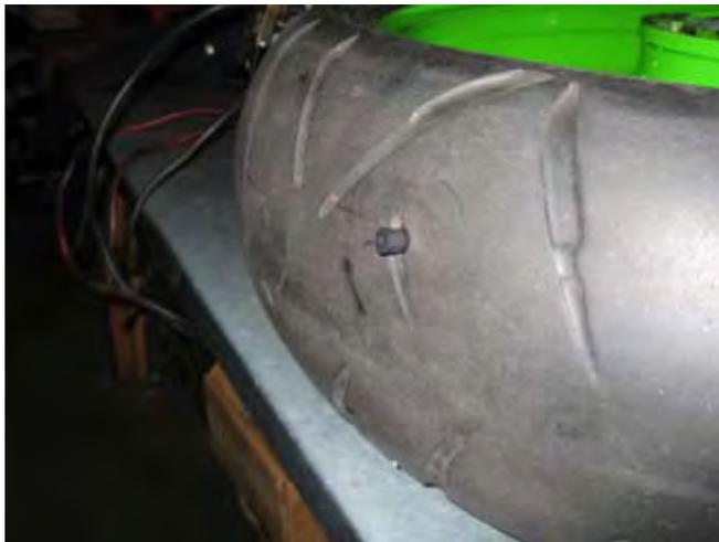
Inflating the tire using the CO2 cartridges was a little more difficult. The venturi effect from the escaping CO2 gas super cools the cartridge, and it's kinda freaky. We inflated a completely empty 190 rear, and the 4 cartridges only netted us 18 PSI.
