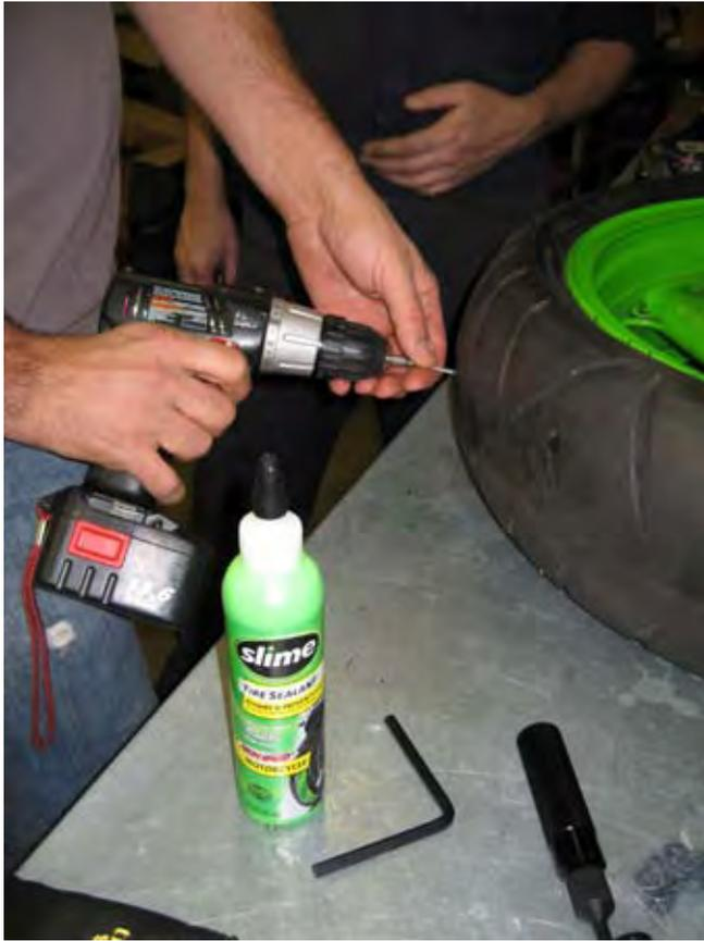
The cap on the Slime bottle has an ingenious valve core-removing tool built into it.
