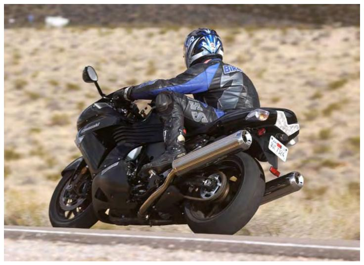
big in diameter the ZX-12R's stock canister was? Emissions standards have changed, and engineers told us that to meet Euro3 spec the can would be so large it would be ridiculous. That accounts for the majority of the extra pounds.
